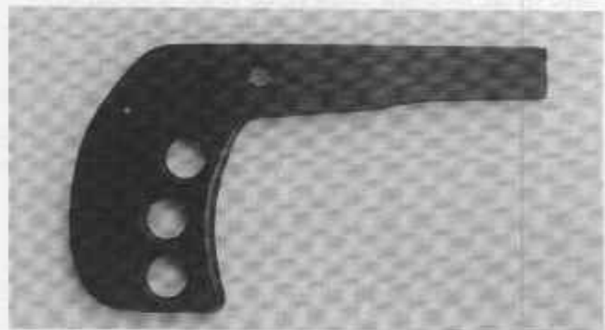
PHOTO 42: The trigger with all holes drilled.
